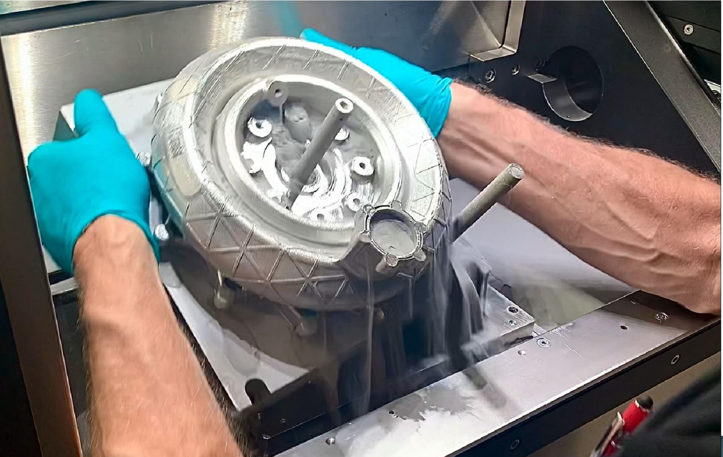
Part: Keselowski Advanced Manufacturing Turbopump Nozzle Material: 718 Inconel Printed On: EOS M290
